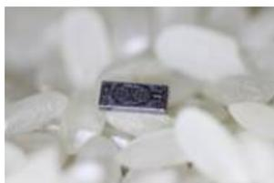
"Caltech engineers developed a new optical gyroscope that is 500 times smaller than the current state-of-the-art device, yet they can detect phase shifts that are 30 times smaller than those systems."
