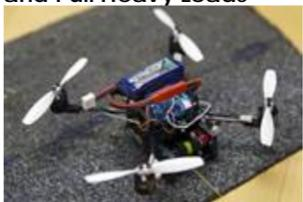
"Small flying robots can perch and move objects 40 times their weight with the help of powerful winches and two previous inventions – gecko adhesives and microspines."
