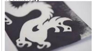
"In research recently published in Science Advances, the group reports on a method for spraying invisibly thin antennas, made from a type of two-dimensional, metallic material called MXene, that perform as well as those being used in mobile devices, wireless routers and portable transducers."
