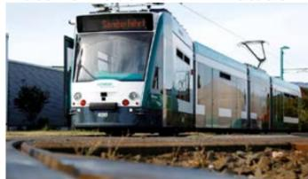
"Fitted with multiple radar, lidar (light from a laser), and camera sensors, forming digital eyes that film the tram and its surroundings during every journey, the tram reacts to trackside signals and can respond to hazards faster than a human."
