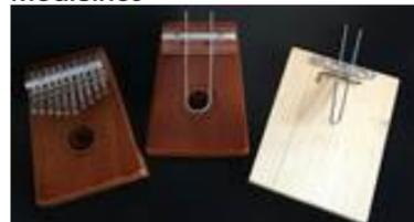
"An inexpensive, handheld tool inspired by an ancient African instrument called an mbira, or thumb piano, can distinguish between liquids of different densities. That could help pharmacists and consumers identify counterfeit and contaminated drugs, which make up an estimated 10.5% of all medications in low- and middle-income countries."
