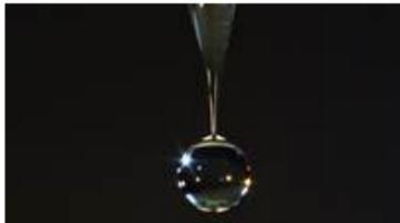
"Harvard University researchers have developed a new printing method that uses soundwaves to generate droplets from liquids with an unprecedented range of composition and viscosity. This technique could enable the manufacture of many new biopharmaceuticals, cosmetics, food and optical materials."
