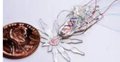
"A new fabrication process enables the creation of soft robots at the millimeter scale with features on the micrometer scale as shown here with the example of a small soft robotic peacock spider with moving body parts and colored eyes and abdomens."
