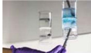
"A team of researchers created a sponge-like material, left, from wood pulp and small bits of metal that can remove color from dyes in water within seconds."
