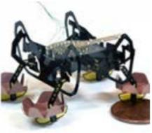
"Harvard's Ambulatory Microrobot, known as HAMR, can walk on land, swim on the surface of water, and walk underwater for as long as necessary, opening up new environments for this little bot to explore."
