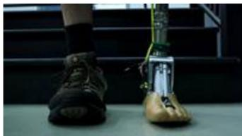
Unlike traditional prosthetic limbs that absorb shocks passively, this prosthetic ankle leverages on sensors, actuators and motors for motion detection and better assistance to its wearer while walking up and down stairs.
