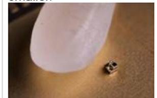
Researchers in the US have come up with the world's smallest computer which serves as a precision temperature sensor. It may also find its place in biomedical diagnosis, surveillance, and oil reservoir monitoring.
