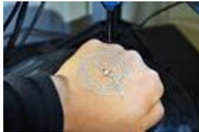
A new 3D printing technique that draws precise patterns of electronic device temporarily onto the skin. Unlike traditional 3D printers, this device makes it possible to print on moving objects.
