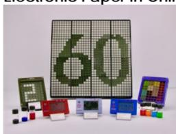
Electrowetting techniques were used for greater colour video e-paper display performance with ultra-fast video streaming, distinct contrast ratio, low power consumption, high resolution and full colour.
