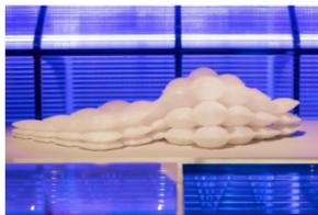
MIT's new [3D printing](#) technology is able to print liquified materials into complex structures with clusters of inflatable and deflatable air chambers. These flexible structures could lead to fully customisable car interiors.
