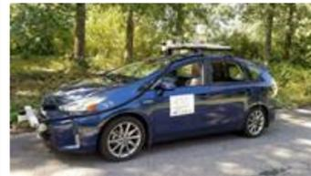
Check out how MIT CSAIL's MapLite enables driver-less cars to navigate with just GPS and sensors, going beyond the driving with exact 3D positions of lanes, curbs, off-ramps and stop signs.
