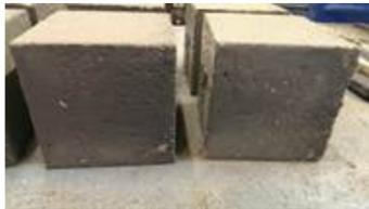
A technique of adding graphene into concrete makes the new material four times stronger and more water resistant while increasing durability by two times and sustainability.
