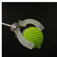
Harvard researchers developed a new type of conductive ink which can be 3D printed into sensors embedded within soft robots, enabling the robots to sense and respond to their surroundings. Read more also at [Advanced Materials](#).
