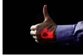
This devices fits snugly on the skin and can show the moving waveform of an electrocardiogram recorded by a breathable, on-skin electrode sensor. Also read about [motion sensors that track stroke survivors](#).
