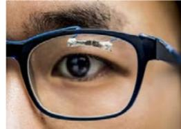
This disposable and wearable sensor made from toilet tissue can detect a person's pulses, blinks of an eye and even heartbeats.
