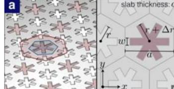
A new sonic insulator that is thinnest ever designed with snowflakes-shaped holes, aims to overcome the vibration-bending boundary and spread out waves. Read more at [APS](#).
