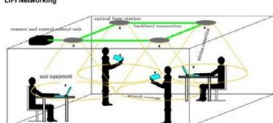
Imagine lights becoming the access points for wireless networking. The 5th Generation wireless technology LiFi uses visible light communication to achieve high speeds of 8 Gbps that is secure, bi-directional and fully networked.
