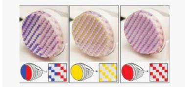
MIT ColorFab develops [a 3-D-printable photochromic system](#) that allows colours to change after 3D printing them. The colours can be activated using ultraviolet light and deactivated using visible light.
