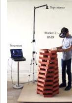
With the integration of Augmented Reality (AR), free-form modular designs can now be constructed by anyone with just AR goggles and a control subsystem, instead of relying on advanced digital fabrication technologies.
