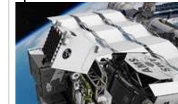
X-Ray based millisecond pulsars are used to pinpoint an object travelling in deep space. The proposed SEXTANT system could find its place in future deep space navigation.
