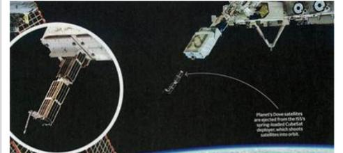
CubeSats, a new kind of miniaturized satellites that are lightweight and low-cost, can outperform the traditional spacecraft when in clusters in terms of the scope of coverage and timeliness of data collection.
