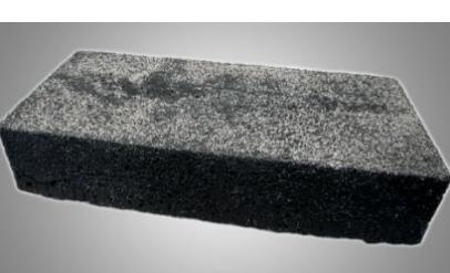
"A new building material developed by engineers at Worcester Polytechnic Institute could change how the world builds. Made using an enzyme that turns carbon dioxide into solid minerals, the material cures in hours and locks away carbon instead of releasing it. It's strong, repairable, recyclable, and far cleaner than concrete. If adopted widely, it could slash emissions across the construction industry."
