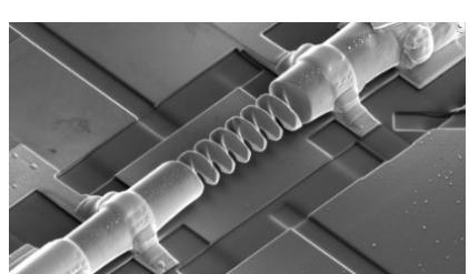
"Researchers have developed a technique that allows them to carve complex three dimensional nanodevices directly from single crystals. To demonstrate its power, they sculpted microscopic helices from a magnetic material and found that the structures behave like switchable diodes. Electric current prefers one direction, but the effect can be flipped by changing the magnetization or the twist of the helix. The findings show that geometry itself can be used as a tool for electronic design."
