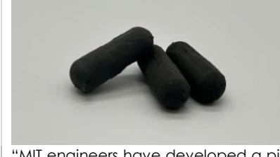
"MIT engineers have developed a pill that can wirelessly report when it's been swallowed. Inside the capsule is a biodegradable antenna that sends a signal within minutes of ingestion, then safely dissolves. The system is designed to work with existing medications and could help doctors track adherence for high-risk patients. Researchers hope it will prevent missed doses that can lead to serious health consequences."
